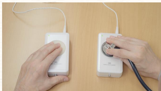
The pulse is output from the left side and the heart sound is output from the right side.
